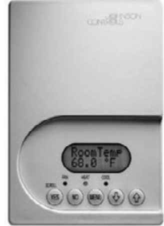
Optional Auto-Variable Speed Thermostat Surface Mounted 3.5" W x 5" H x 1.25" D Requires 4 Low Voltage Conductors
