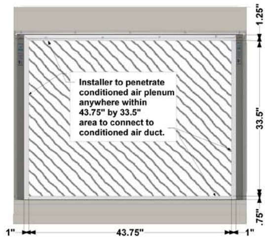
Conditioned Air Plenum View
