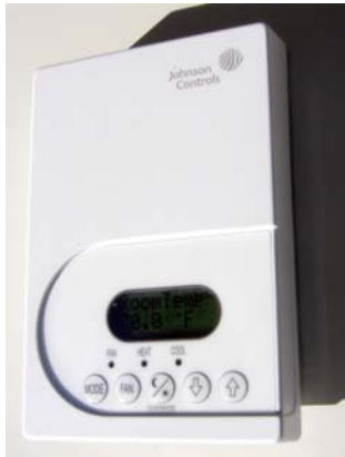
Auto-Variable Speed Thermostat Surface Mounted – 3.5" W x 5" H x 1 1/4" D Requires 4 Low Voltage Conductors
