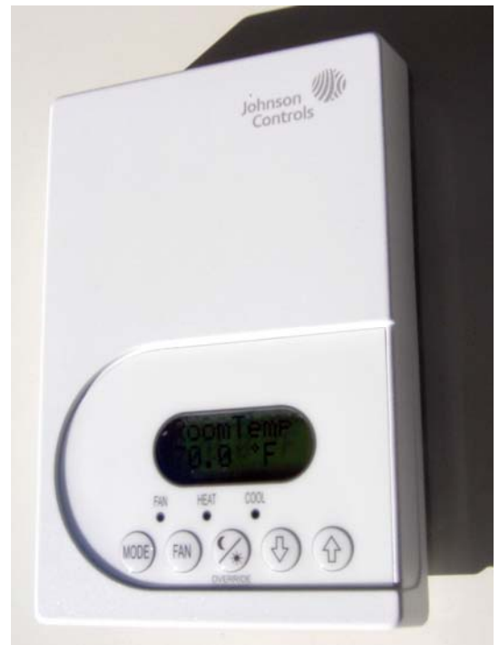
Optional Auto-Variable Speed Thermostat Surface Mounted – 3.5" W x 5" H x 1¼" D Requires 4 Low Voltage Conductors
